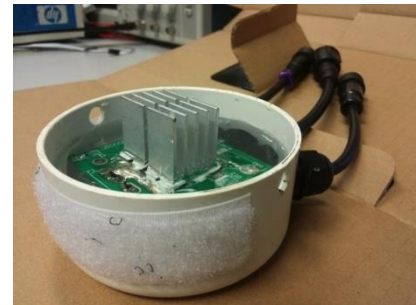
Figure 16: Waterproofed motor driver
