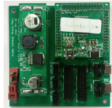
Figure 14: The Octopus's control unit, with core board, extension board, and regulator board designed by our hardware team
