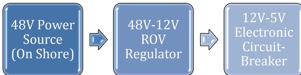
Figure 7: Power delivery system for the Octopus ROV
