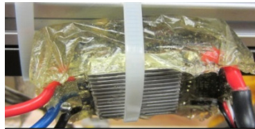
Figure 11: Epoxy-potted speed controller
