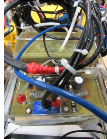
Figure 4: Epoxy-potted Arduino Mega (translucent block at top of image)
