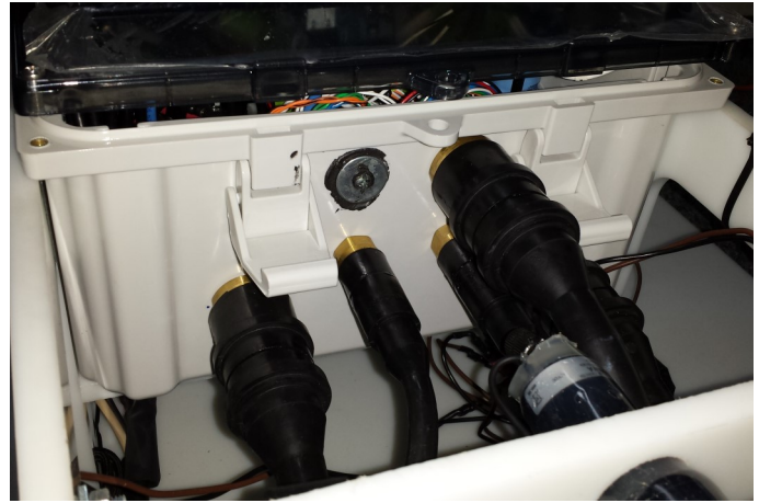
Figure 13—Several SubConn bulkheads securely mounted to the main dry housing
