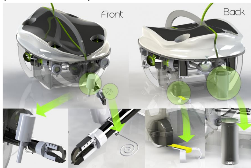
Figure 18. Conductivity sensor, spiral hook, tape and sampler (CAD model)
