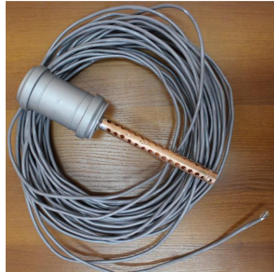
Figure 16. Conductivity sensor (scheme and real assembly)
