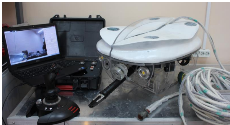
Figure 2. ROV "Alien Ghost" with surface equipment
