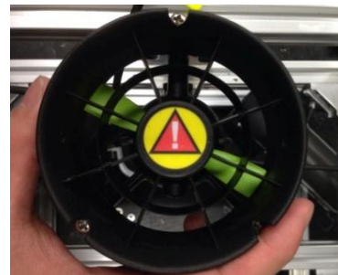
Caution marks on the hood of the thruster
