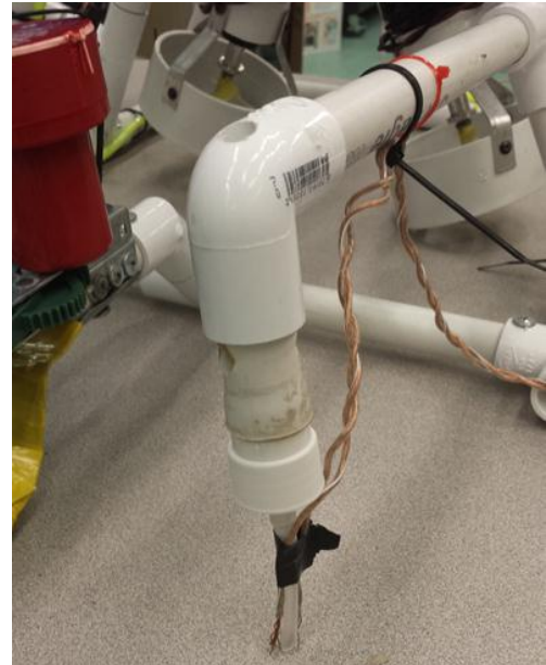
Agar Extractor with conductivity wires at tip
