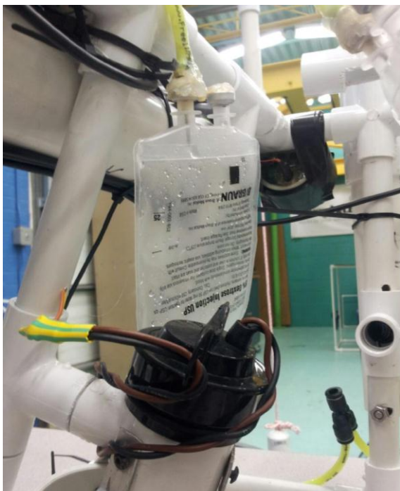
Buoyancy Control Air pouches
