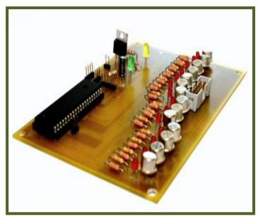
Figure 2 PIC Control Circuit Board
