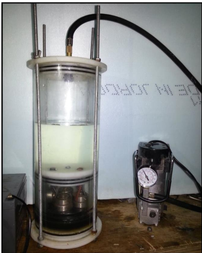
Figure 48 The pressure chamber used to test components.
