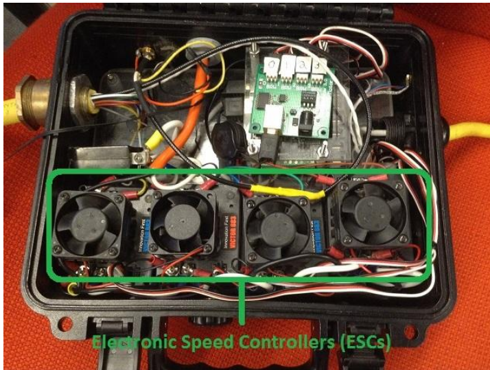
Figure 18: Electronics Control box
