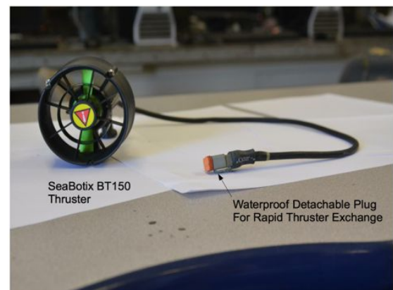
Figure 5. SeaBotix BT150 with rapid exchange connector.
