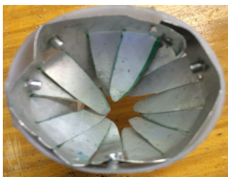
Figure 8. Core catcher prototype.
