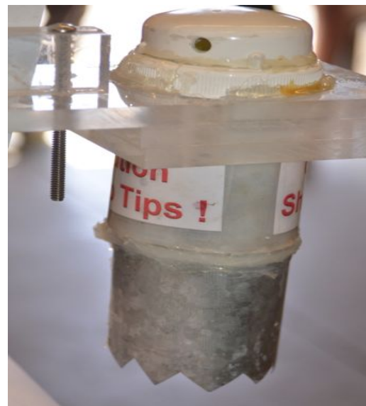
Figure 7. Bacterial mat sampling device
