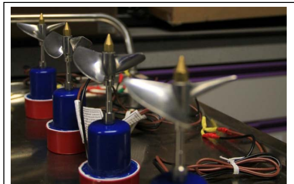
Fig.1 Our modified bilge pumps as propeller driver
