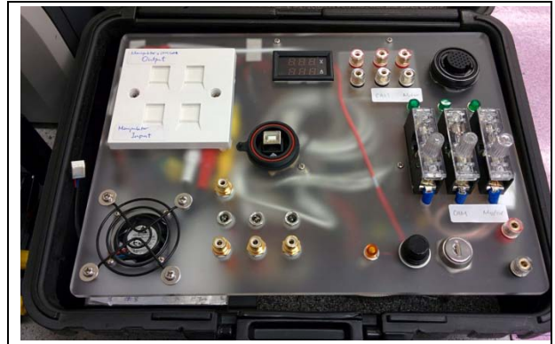
FIG. 4 QUICK FIT POOLSIDE ELECTRONICS BOX
