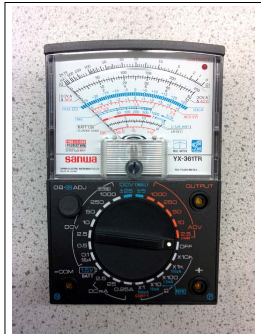
FIG. 16 SANWA YX361TR ADAPTED FOR CONDUCTIVITY SENSOR
