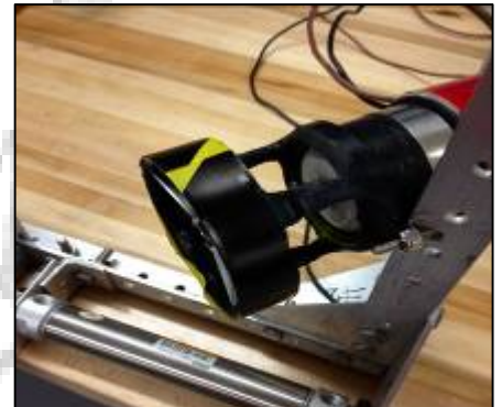
Shrouded bilge pump with warning tape (T.R.)
