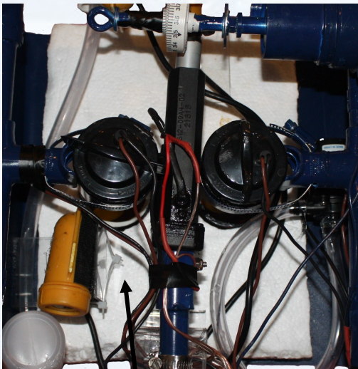
Closed cell foam in the center of the ROV frame.
