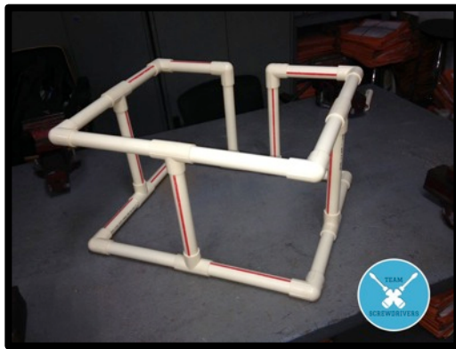
Fig 3.1 PVC Pipes Chassis
