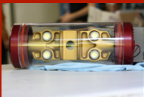
Image 5-7: LED lights for diver visibility and warning labels around moving parts are clearly indicated.
