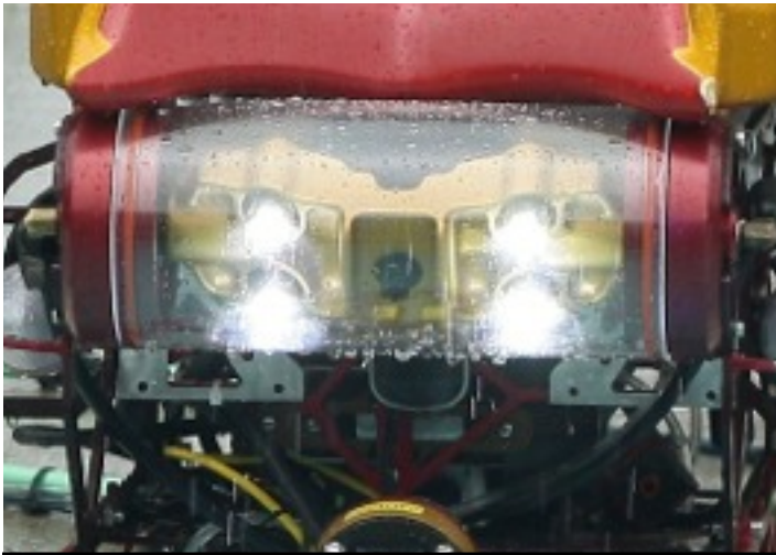
Image 20: Rotating camera assembly with HD wide angle camera and four LEDs.
