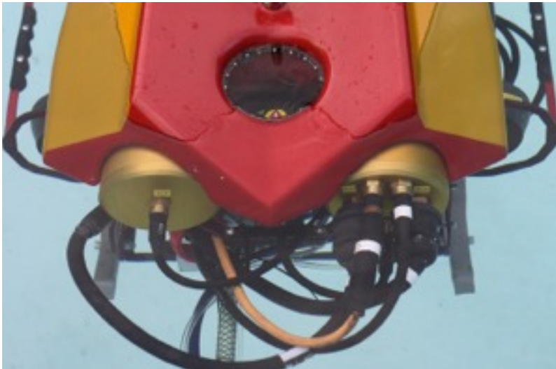
Image 19: SEA CON and Sub-Con connectors make individual components and the tether detachable from \Sigma VII.
