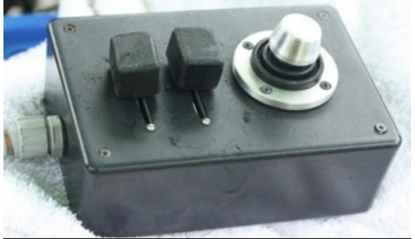
Image 17: Human interface controller for ROV's thrusters and rotating camera assembly.
