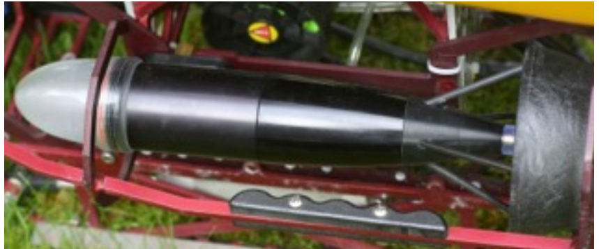
Image 14: One of the two VideoRay thrusters that provides the horizontal movement for \Sigma VII.
