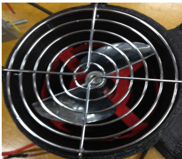
All of the motors are completely encased and covered by fan guards.
