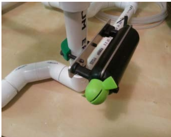
Figure 5: Thruster mount with prototype round clamp (in green)
