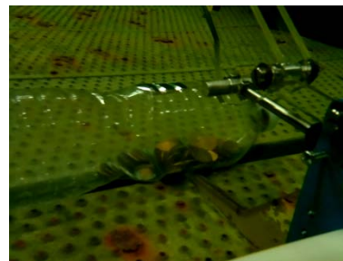
Figure 21: ROV grabbing a water bottle on the tank floor
