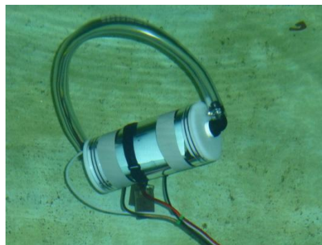
Figure 17: Picture of the electronics enclosure being water proof tested
