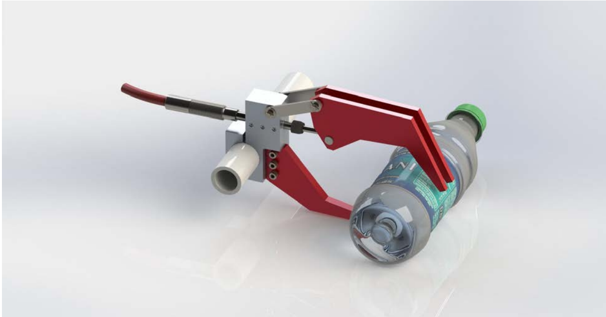
Figure 9: CAD picture of the functioning claw design grabbing a water bottle
