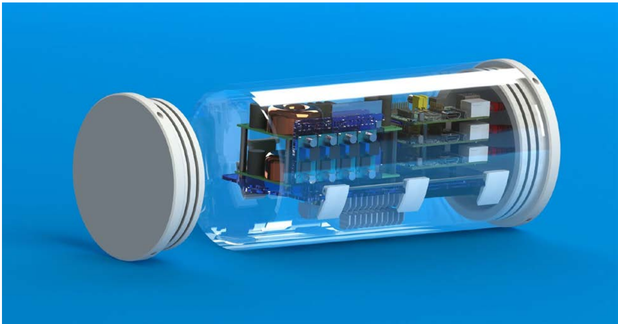
Figure 10: Picture of our electronics enclosure made from 6 inch acrylic tube with all the electronics neatly mounted inside the tube
