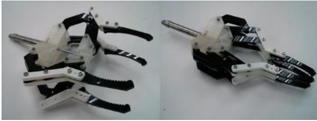
Figure 16: Open/Close state of manipulator
