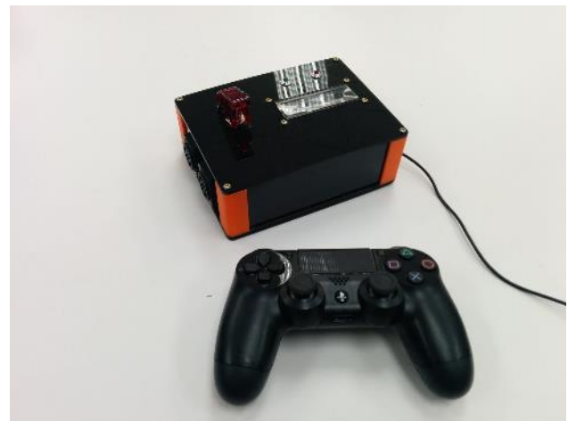
Figure 5: On-shore/surface control box
