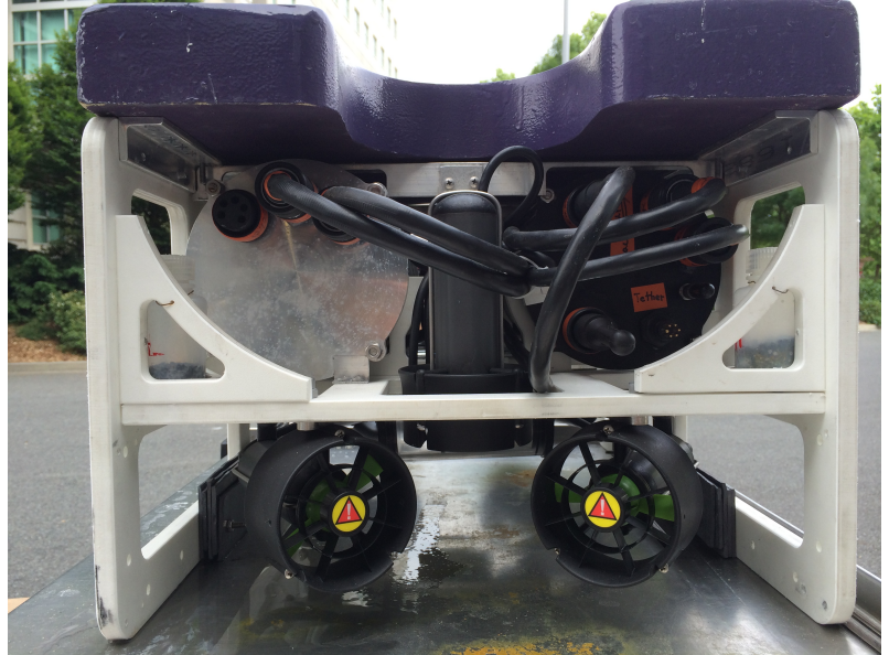
Fig. 2. Back view of ROV with motors displayed on the bottom and pressure housings encased above.
