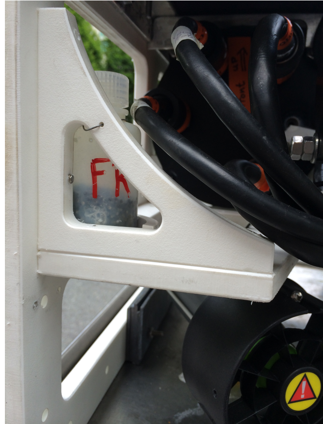
Fig. 6. Bottle with lead pellets located in the corner and lead strips bolted to the inside bottom edge of the ROV frame.
