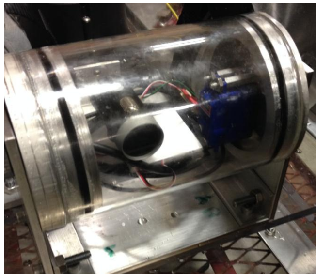
Figure 13: O-rings and marine grease were used to seal the end caps of the various electronics tubes.
