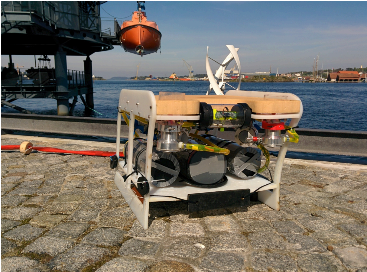
Njord the ROV without the manipulator mounted.
