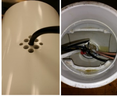
(a) How the tether was mounted into the buoyancy vessel
