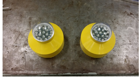
Figure 4: The headlight fixtures
