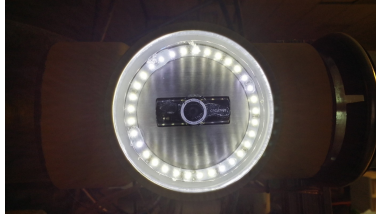
(b) The side view camera, showing the ring leds
