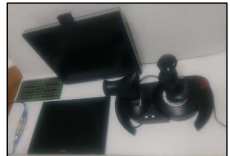
Fig. 32: Control station prototype
