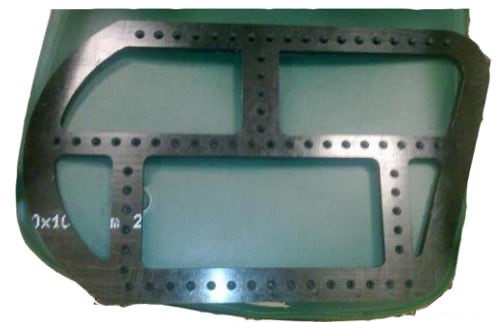
Figure 3: Black polyethylene body Frame
