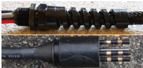
Figure 7: Top: a potted cable gland; Bottom: a female bulkhead (Credit: R. Miller)
