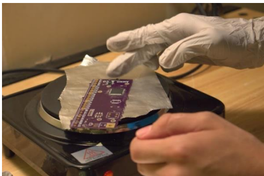
Figure 21: Using a hot plate to solder a miniscule Arduino chip onto a custom PCB, with gloves for safety (Credit: A. Miller)
