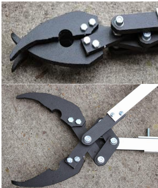
Figure 17: The manipulator closed (top) and open (bottom) (Credit: A. Miller)
