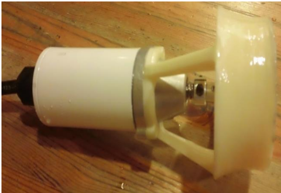
Figure 10: The completed thruster assembly (Credit: C. Orndorff)
