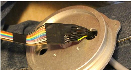
Figure 15: The remote programming cable with the WEC's front end cap (Credit: A. Miller)
