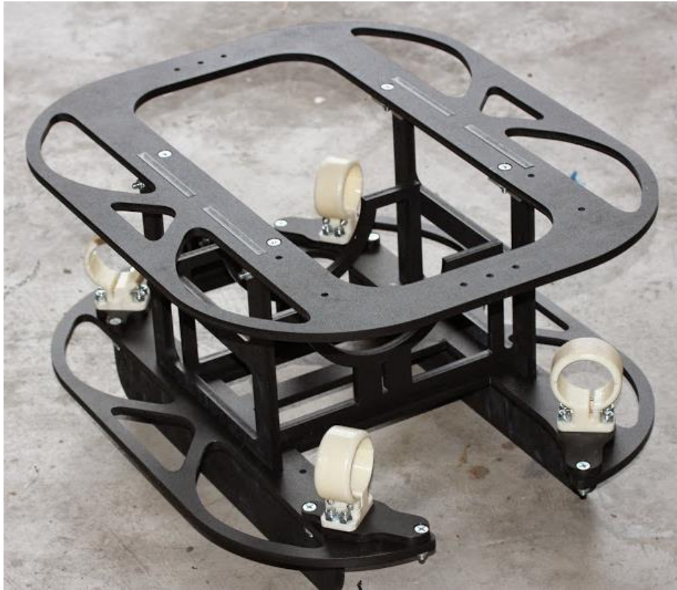
Figure 5: The frame with four of the 3D-printed thruster mounts (Credit: A. Miller)
