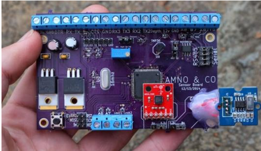
Figure 13: The assembled PCB for sensor control (Credit: A. Miller)
