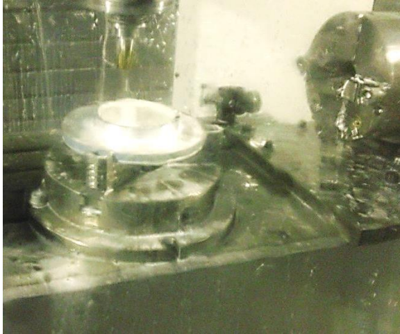
Figure 26: Partway through the machining process of one of the WEC end caps (Credit: C. Orndorff)
