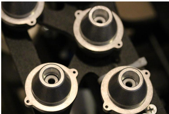
Figure 9: Several of the end caps immediately after machining (Credit: R. Miller)
