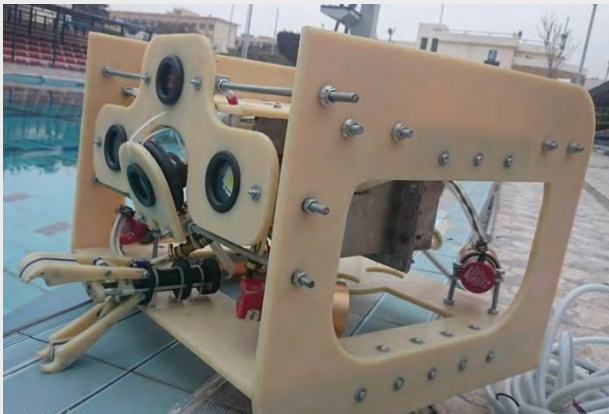
Figure [15] Initial assembly - Before applying Foam & Fiberglass
