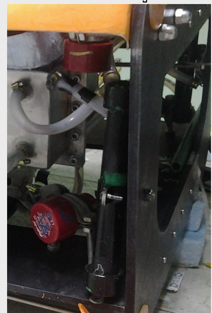
Figure [13] Creating Balancing system by adding ballasts to the vehicle corners
