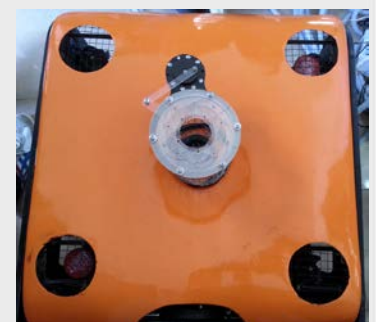
Figure [35]. Sample Catcher fixed above the top camera
