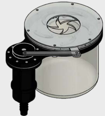
Figure [34]. Sample Catcher 3D CAD model
