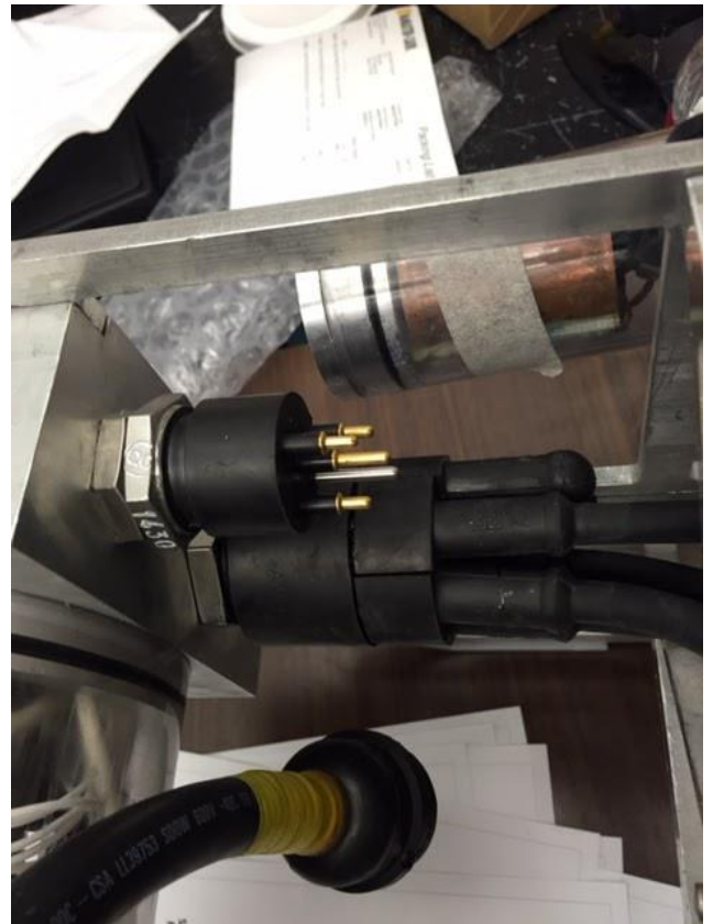
Fig. 8: The 24-pin pie connector, with multiple male connectors feeding into a single female connector. This allows for rapid swapping of motors and a more intuitive design.
