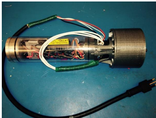
Fig 6: Motor Enclosure with Propeller Cowling on the front
