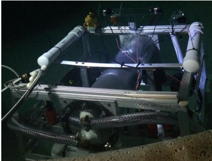
Figure 4. The ROV during a night test, before we balanced it with the right buoyancy and ballast. At this point, it was neutrally buoyant and stayed at this off-kilter position for almost 45 minutes. However, driving the ROV is difficult when it constantly leans.
