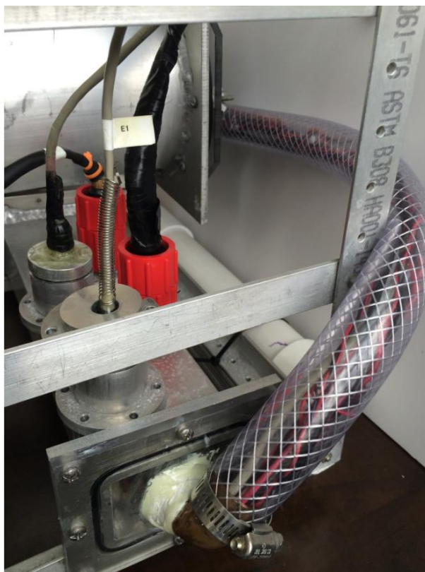
Figure 6. The custom aluminum ethernet connectors, and red SubConn connectors on the secondary connector box. The end of the box shows the tube routing wires from this half through to the main canister, where they connect to the electronics.
