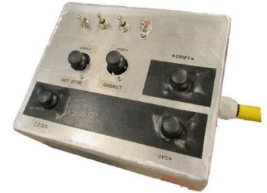
Figure 4: Custom Control Box Consists of a Phidget 8/8/8 board, Joysticks, and analogue switches.
