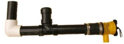
Figure 28: The Vacuum - Collects algae.
