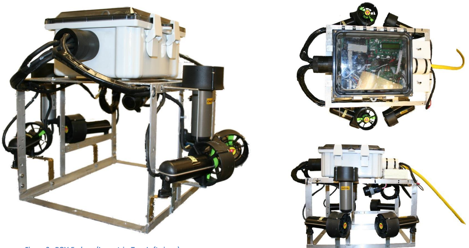
Figure 2: ROV Erebus . (Isometric, Top, Left views) Isometric (left), Top view (top right), Left view (left-bottom)
