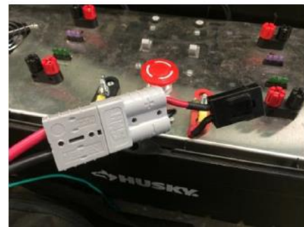
Figure 26: Quick disconnect in line 20A fuse holder.
