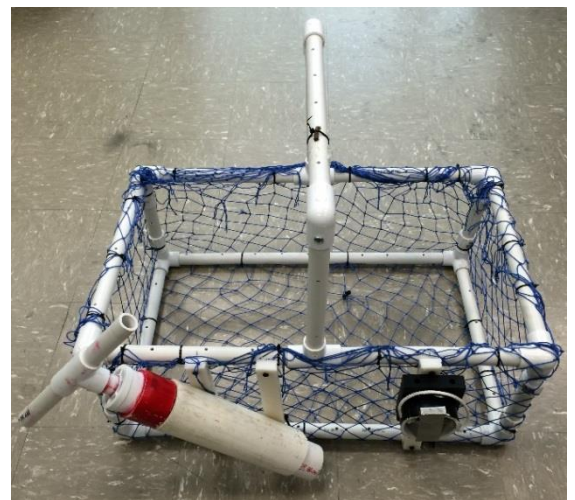
Figure 22: Tool basket with hot stab and wellhead gasket.
