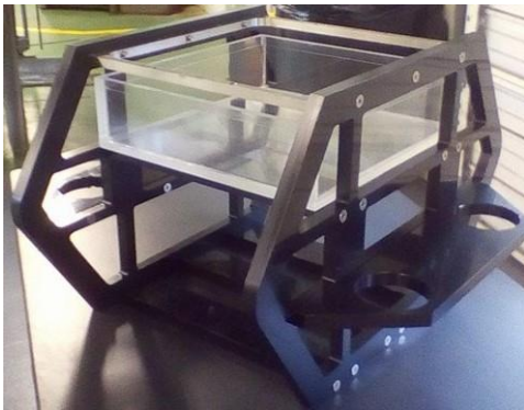
Figure 2a: HDPE frame with acrylic ebox.
