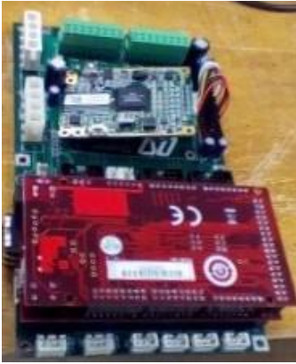
Figure 10a: A top view of the Low Voltage Control Board designed by our Electronics Engineer.
