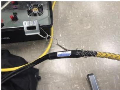
Figure 25: Strain relief hook attached to tether and power supply
