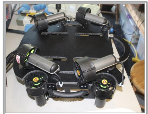
Figure 6: Configuration of the thrusters. The four thrusters on top are the vector thrusters and the four thrusters at the bottom (only two visible in this figure) are used for vertical movement.
