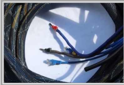
Figure 13: Tether and surface connectors
