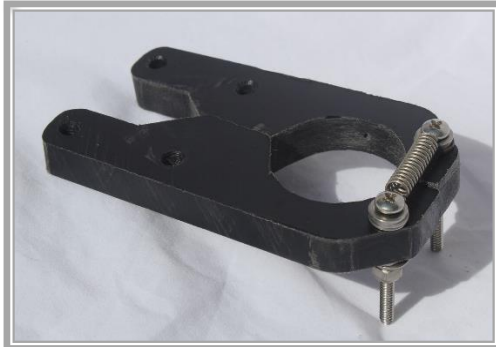
Figure 11: One of the clamps that make up the lift line. This holds the 1-1/2" PVC pipe.
