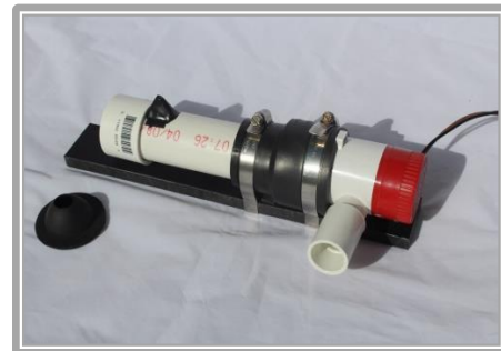
Figure 10: Vacuum pump and rubber fitting
