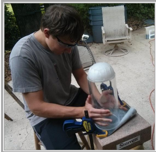
Figure 5: Oscar sands the bottom of the canister to provide a better seal.
