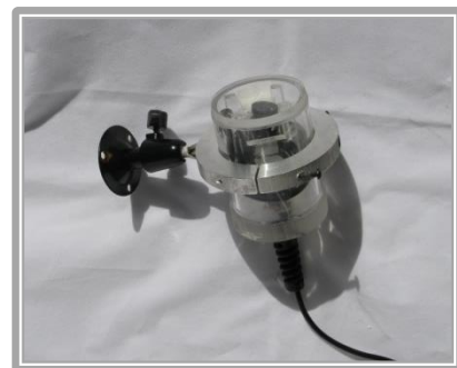
Figure 19: The Vega's camera and clamp
