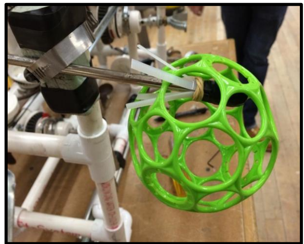
Figure 9: Pictured above, the zip-tie spear securing the sea urchin.
