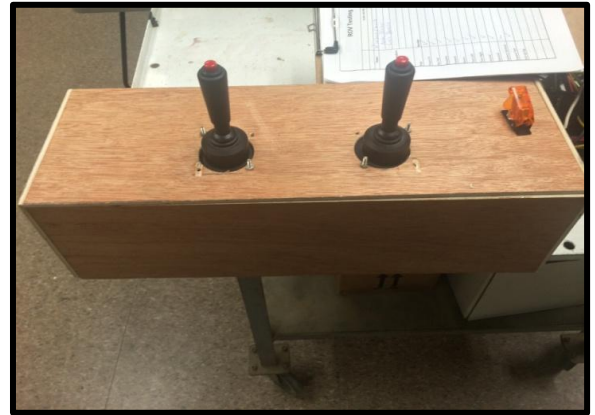
Figure 12: The control box for The Black Pearl , above.
