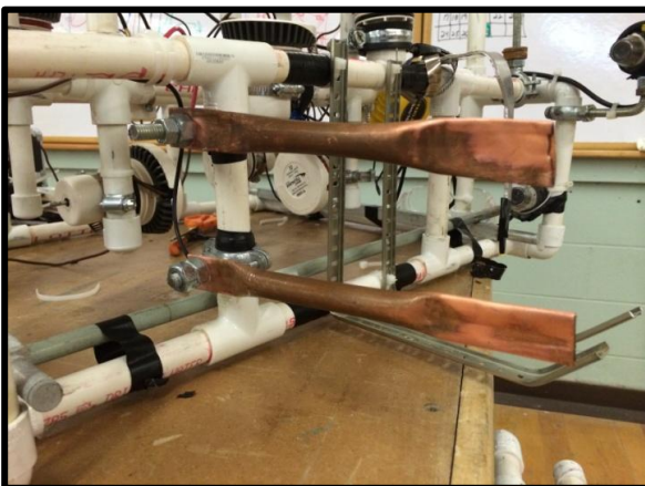
Figure 10: The copper anode testing mechanism.
