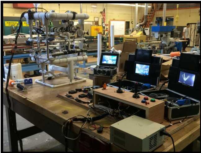
Figure 21: The completed ROV on its stand with the three monitors displaying camera views is shown above.
