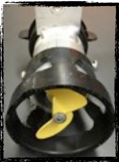
Fig. 4- The aluminum mount and ABS shroud attached to a bilge pump motor.
