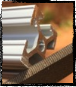
Fig. 19- All edges of the frame's aluminum extrusion were filed down.
