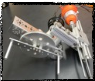
Fig. 13- Valve Rotator with orange paint on the motor, indicating that it is a moving part.
