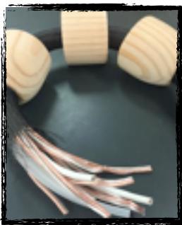
Fig. 9- The cables within the PET covering with handmade wooden buoys.
