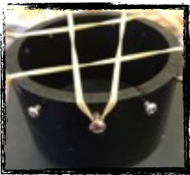
Fig. 14- Algae Collector with rubber bands on the screws to capture the ball.
