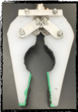
Fig. 12- Plastic gripper with liquid and rubber tape for grip.
