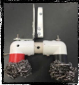
Fig. 15- Voltage Tester that uses stainless steel wool to measure voltage.
