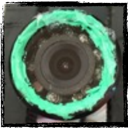
Fig. 8- The Through Hole cameras were waterproofed with green liquid tape and clear RTV silicone.
