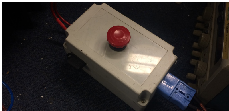
Figure 11: Emergency kill box with inline fuse
