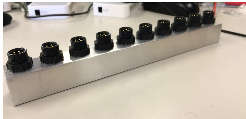
Figure 14: The main CAN bus hub
