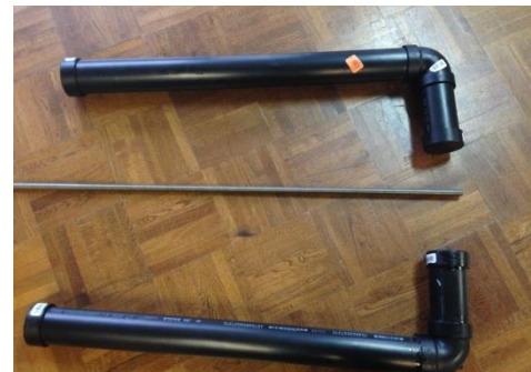
BUOYANCY TANKS AND REBAR BALLAST
