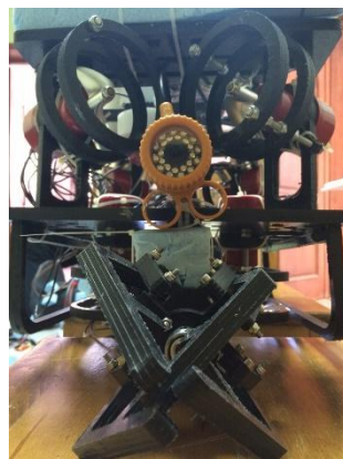
Figure 3 showing the ROV's front assembled and tested with one front arm
