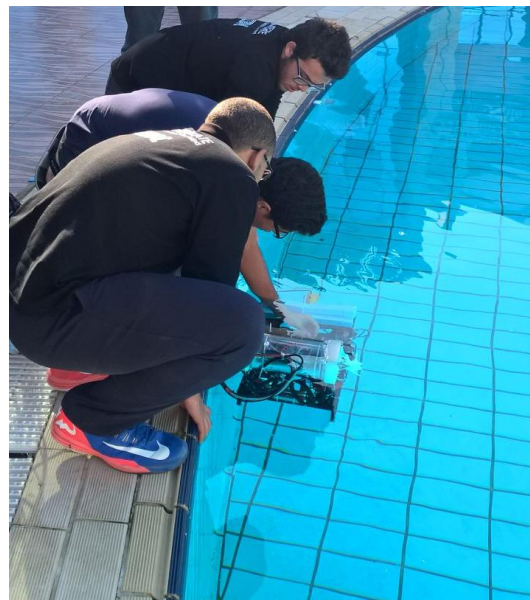
Figure 17 Integrate Orca team adjusting the buoyancy of the ROV.
