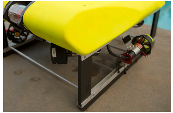
Figure 5. Stingray's front pair of 45° thrusters with a side-mounted thruster.
