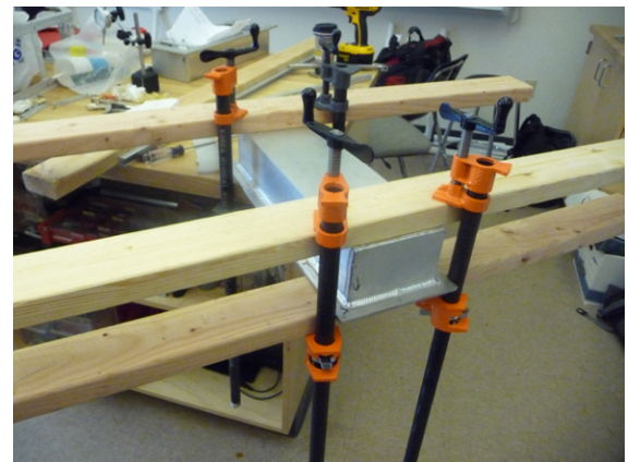
Figure 30. Wooden framework ready to bend the electronics housings into the correct shape.
