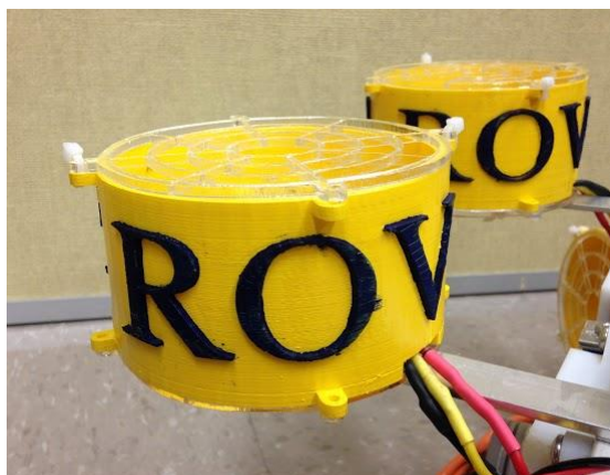
Fig. 12 Custom 3D printed thruster shrouds for enhanced safety.
