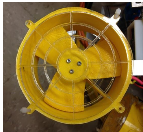
Fig. 11 LBCC ROV proprietary 3D printed propellers with empirically tested blade pitch to maximize thrust.
