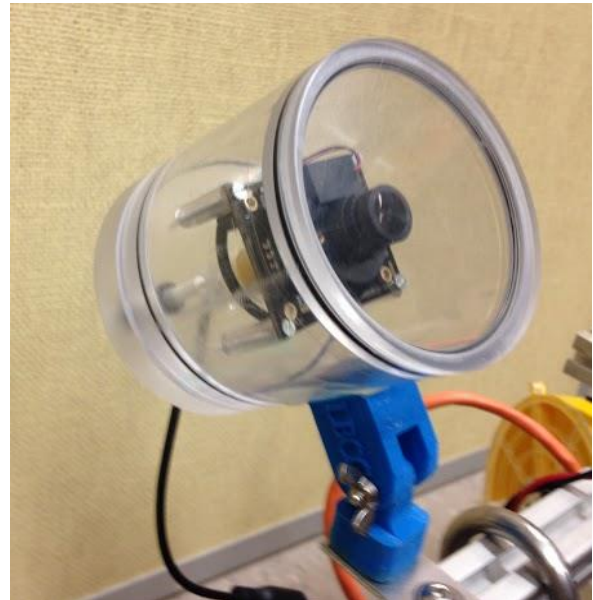
Fig. 13 One of the Water Bear's cameras including its housing and mount.
