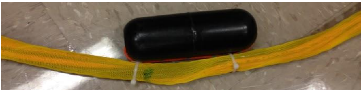
Fig. 14 Section of the Water Bear's tether including a floatation buoy
