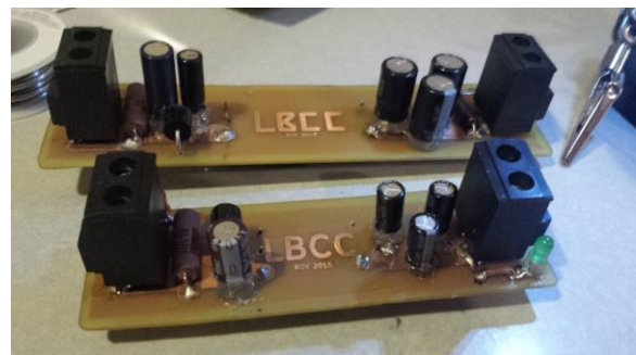
Fig. 9 Arm and camera power boards before epoxy.
