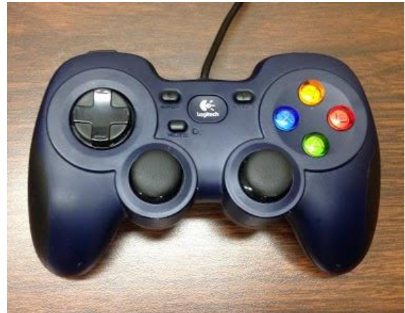
Fig. 7 USB Logitech game controller used for maneuvering the Water Bear.
