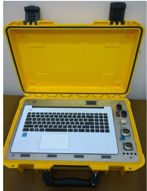
Figure 14. Control board (with a display removed)
