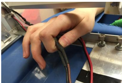
Figure 27 above: Soldered and shrink wrapped wiring. (Credit: Maria Halleran)
