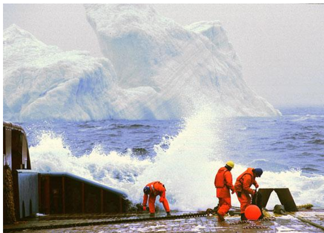
Figure 2: Oil workers in Newfoundland prepare to move an iceberg off its course to prevent it from colliding with Hibernia. Retrieved from: http://mentalfloss.com/article/26994/thin-ice-fight-control-arctic-economy 05-07-15.
