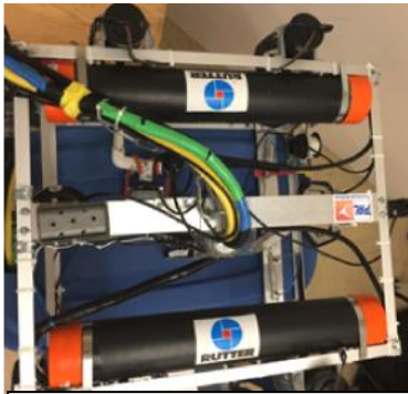
Figure 24: ABS pipe for buoyancy of TMR 1. (Credit: Mitchell Sparkes)
