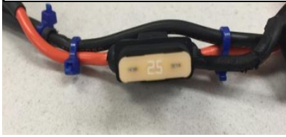
Figure 28: Soldered and shrink wrapped wiring. (Credit: Maria Halleran)
