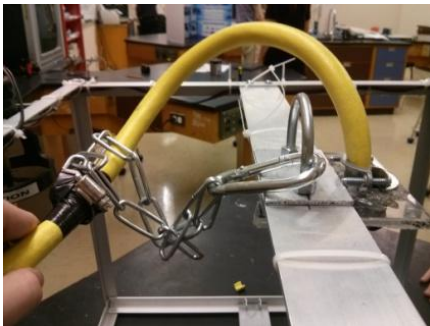
Figure 29: Double strain relief of tether. (Credit: Laura Johnson)
