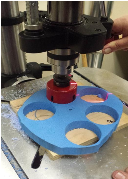
Hole saw cutting buoyancy donuts
