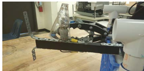
Anode detector covered and attached to ROV
