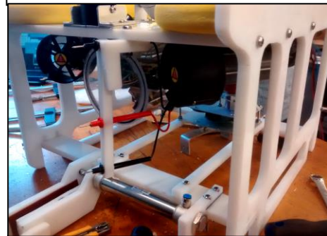
The Regional frame had extra supports; however, these are not present in the final frame. (Photo: A. D.)
