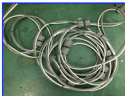
Figure 15 – 12 & 20 core tether cables used for ROV Njord (S.Hope 2015)
