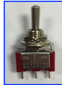
Figure 12 – SPDT switch used to operate the water pump (S.Hope 2015)
