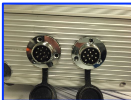
Figure 3 – 12 pin connectors, which make our tether detachable (S.Hope 2015)
