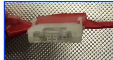
Figure 13 – 25A fuse fitted to the main power connection (S.Hope 2015)
