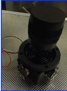
Figure 11 – Joystick, which controls ROV Njord's movements (S.Hope 2015)
