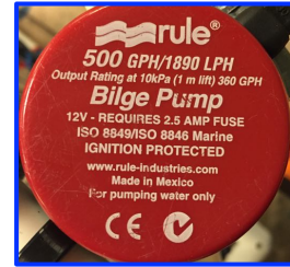
Figure 7 – One of the bilge pumps that equips ROV Njord. (S.Hope 2015)
