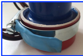
Figure 1 – Jubilee clips protected using heatshrink. (S.Hope 2015)
