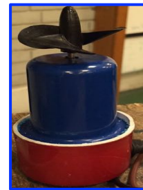
Figure 9 – Modified bilge pump with propeller (S.Hope 2015)
