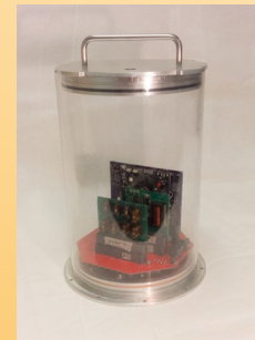
Fig. 6- Electronics Enclosure with electronics inside
