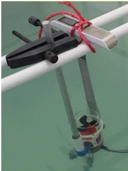
Figure 9. Motor mounted in propeller test arrangement.
