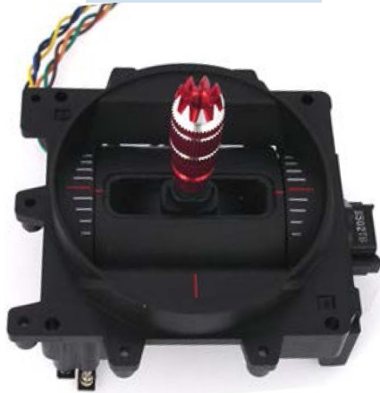
Parallax Inc. Analog Gimbal Joystick used to input pilot movement directions into the Arduino processor board.
