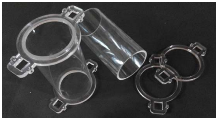
Fig 8. design tube after laser cutting (Rafsi, 2015)
