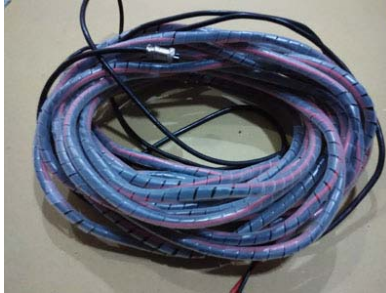
Fig 26. Tether with spiral guard (sabil, 2014)
