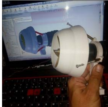
Fig 25. Propeller guard with 3D printing (Rafsi, 2015)
