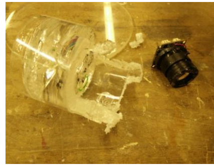
Figure 26 Failure of waterproofing
