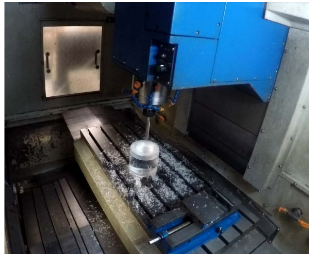
Figure 9: Photo of dome on CNC machine
