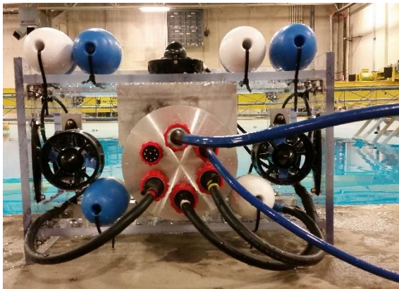
Figure 1: The back view of the final design of the UNH ROV, code named Viper, showing the connections to and from the electronics housing tube as well as the forward/backward thrusters.
