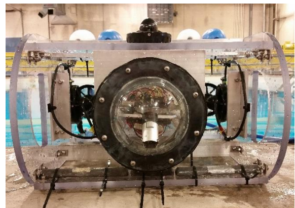
Figure 2: The front view of the final design of the UNH ROV, showing the camera dome as well as the frontal support beams for the mounting of sensors, lighting, and various manipulators.
